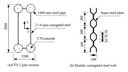
Fig. 4. CFS-2 pier section (dimensions in mm)
