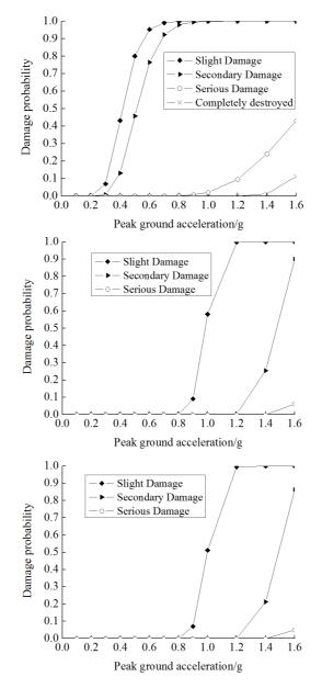
Fig. 7. Comparison of vulnerability curves of three kinds of high piers structures: up–RC pier vulnerability curves, medium–CFS-1-pier vulnerability curves, bottom–CFS-2-pier vulnerability curves
